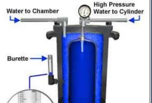
extinguisher's cylinder. As the pressure increases, the cylinder will expand and push water from the steel chamber through a small hole and into the glass burette. After the pressure is released, the cylinder will contract and the water will move from the burette back to the steel chamber. Depending on the results, the tester will either pass or fail the cylinder. The cylinder is normally considered unsafe and will fail if:
